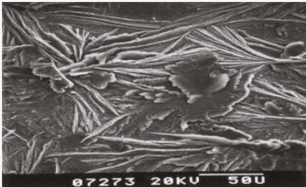
Coating Formation: Effect of Activation on Zinc Phosphate Coating)
