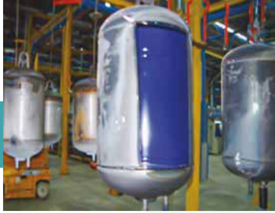
Figure 9. Application of a water heater boiler coated with the plastering method
