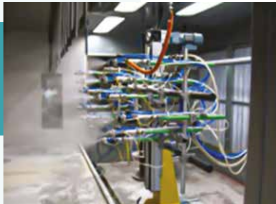
Şekil 8. ESTA uygulama kabini (Referans: https://www.eic-vitreous-enamel.com/equipmentprocess/coating/spraying/electrostatic-wet-enameling.html , 2019)
