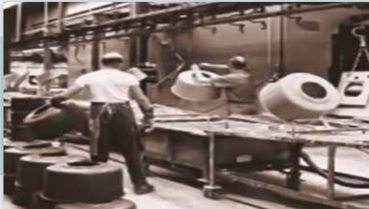
Figure 6. Enamel coating of the washing machine body by immersion method
