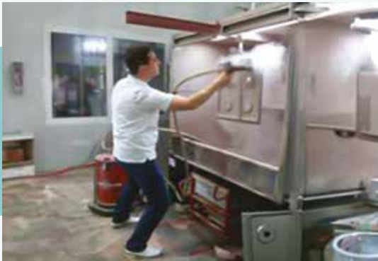
Figure 5. Electrostatic powder enamel application (Artel Uzbekistan enamel plant, 2015)
