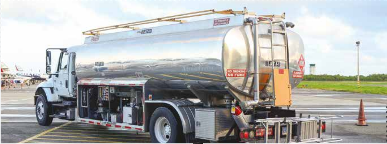
Figure 6: Electropolished tanker for high-purity products transportation [7]
